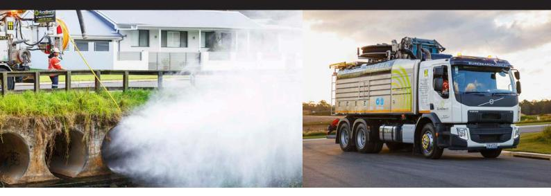
SureSearch has a fleet of combination high velocity drain cleaning trucks are capable of cleaning debris and roots from both storm water and sewer mains ranging from 150mm diameter to 1800mm diameter.
